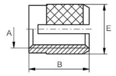
Female thread A = M2,5 Length B = 5.0Min distance to edge = 3.0Outer diameter E = 4.00Recommended bore diameter = 4 to 4.1
